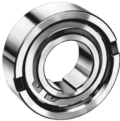
Model ASNU is a ramp & roller type clutch, non-bearing supported. Bearings are required to support axial and radial loads. Lubrication and sealing are required.
